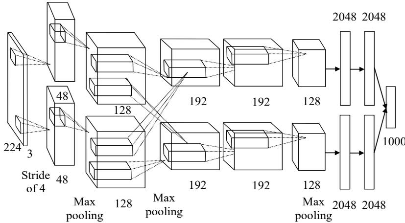
Fig. 1. Architecture of AlexNet 2012 DCNN [21]
