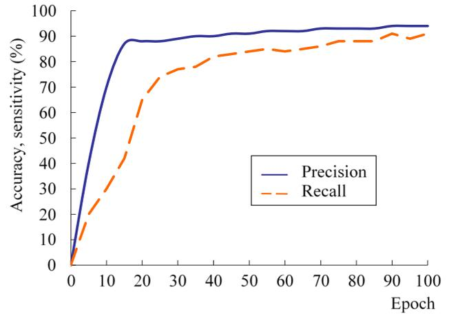
Fig. 15. Graphs of change in the accuracy (precision) and sensitivity (recall) with the test sample depending on the epoch for the proposed AlexVisDrone model
