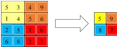
Fig. 3. Max pool operation
