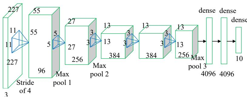
Fig. 2. Architecture of the proposed deep convolutional neural network (base AlexNet 2012)
