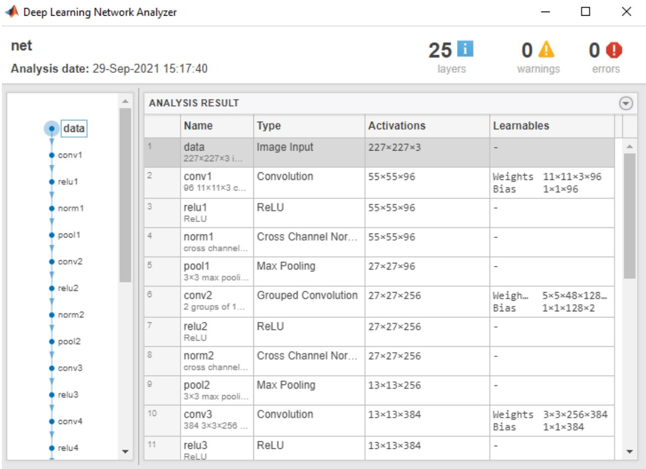
Fig. 11. Visualization of information about AlexNet 2012 network layers using Deep Training Network Analyzer
